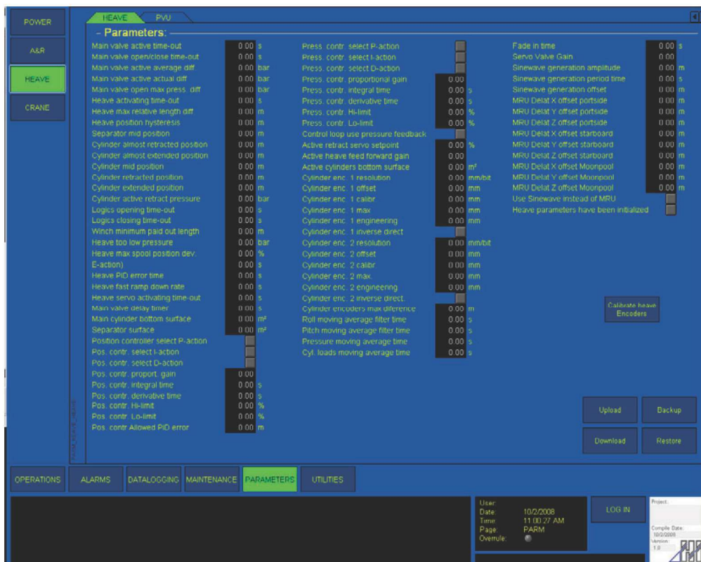
Figure 5-30: PARAMETERS > HEAVE > HEAVE COMPENSATION
