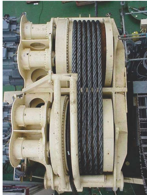
Figure 2-8: Zero fleetangle between drums
