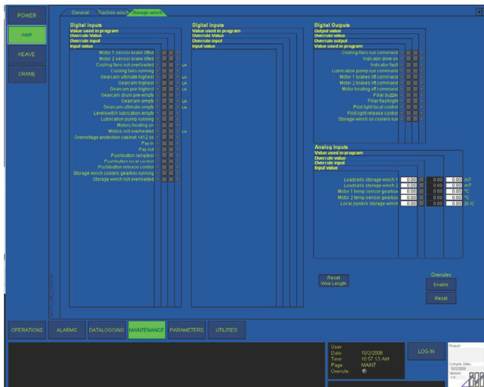
Figure 5-49: MAINTENANCE > A&R > STORAGE WINCH
