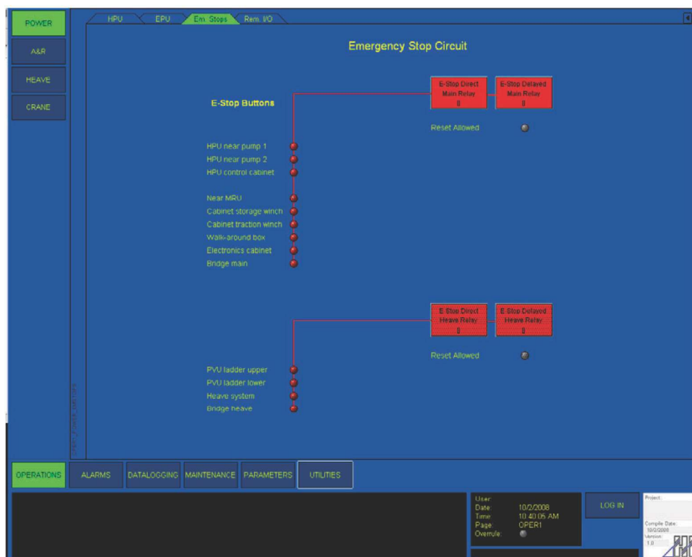
Figure 5-18: OPERATIONS > POWER > EMERGENCY STOPS
