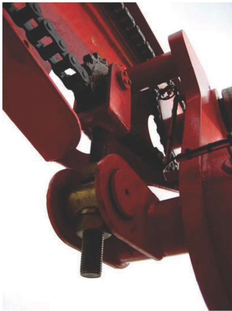
Figure 2-12: Chain tensioner and proximity switch
