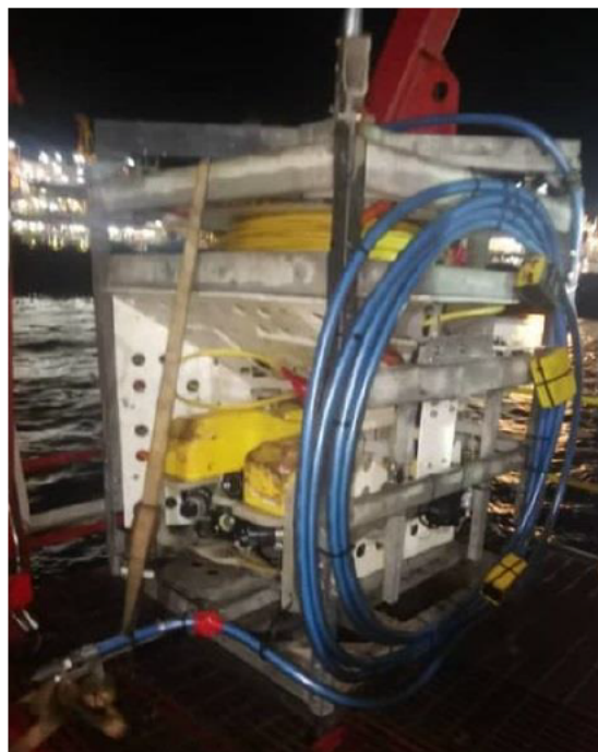
The Seaeye Tiger equipped with high pressure water jetter for jacket member cleaning
