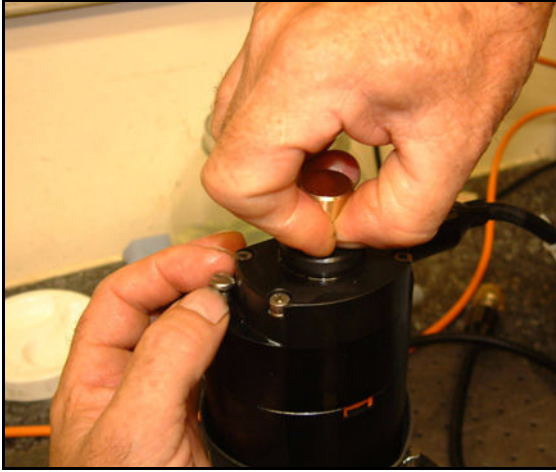
Figure. 7.5 Diaphragm Tool Pin Insertion
