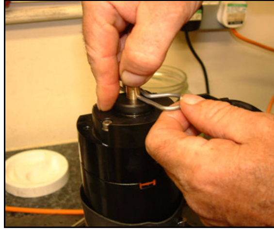
Figure. 7.5 Diaphragm Tool Pin Insertion
