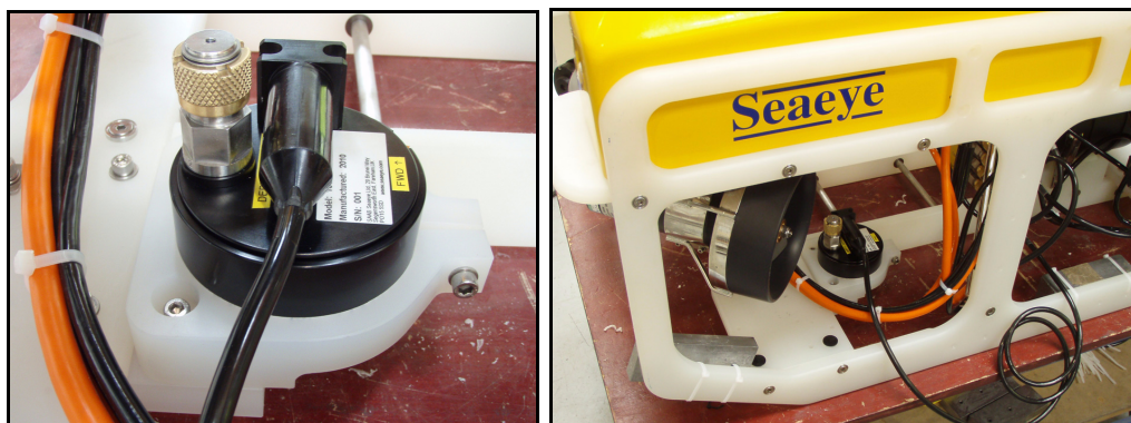
Figure. 1.14 Compass Unit with Depth Unit Socket Connection
