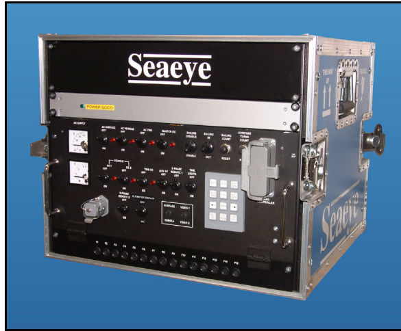
Figure. 2.1 Surface Distribution Unit
