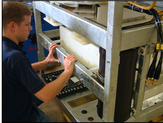
Figure. 6.2 TMS Rear Crossbar Removal
