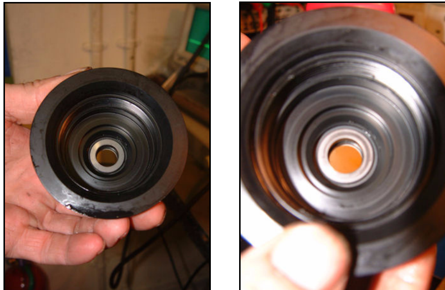
Figure. 6.11 Detail Showing 'Clean' Ceramic Seal and 'Marked' Ceramic Seal
