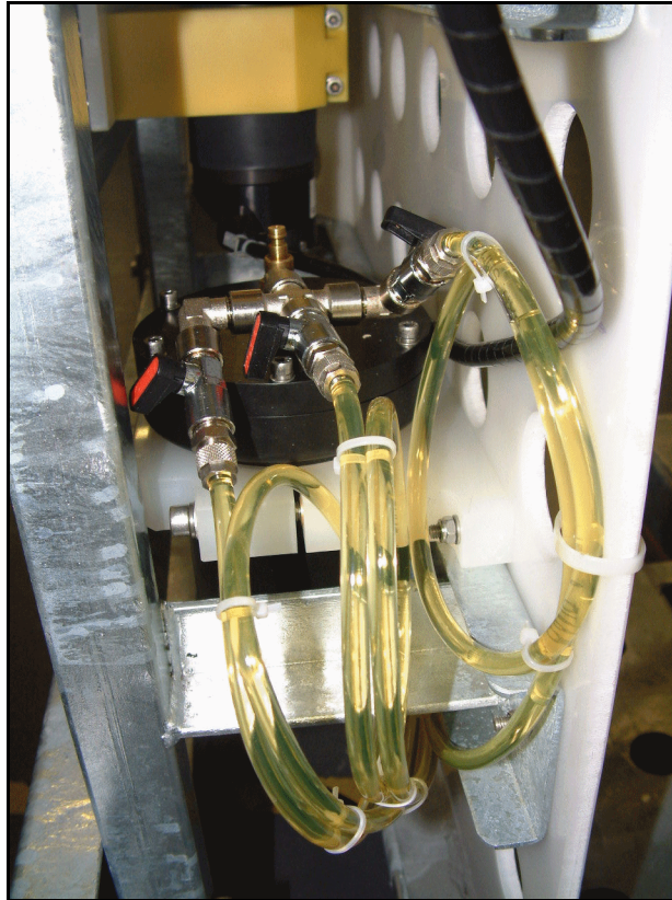
Figure. 7.16 Oil Compensating System
